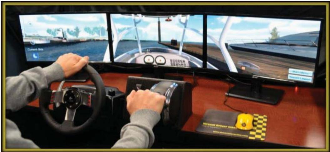
You sit down in front of three computer monitors, a steering wheel, throttles and other controls and perform tasks as you would on the water. The simulation is very realistic especially when you add in wind, currents and day/night scenarios.
